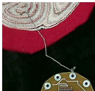
Figure 11.6a, b Back of Musical Jacket keypad with circuit board directly connected to the fabric, by a mechanical/electrical connection made by a knotted yarn.
