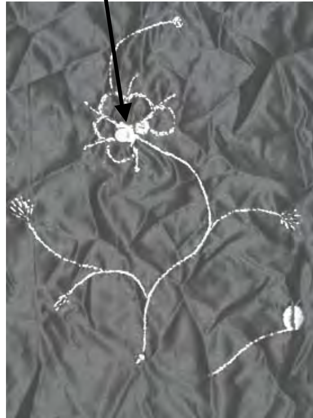
Figure 9.9 An early example of the conductive, floral embroidery, used in the Electronic New Year's Eve Ball Gown .
