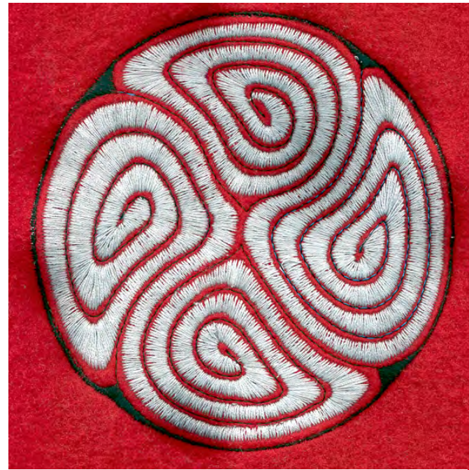
Figure 11.15 Embroidered ground electrode from the Generic Ball .
